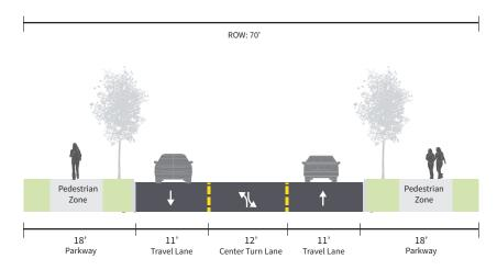
M3U Minor Arterial (70') Note: This cross section is for the frontage road section.
